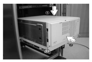
12 Secure the server to the back of the server tray using the two attached screws. To access this location, you may need to open the back door of the rack.
